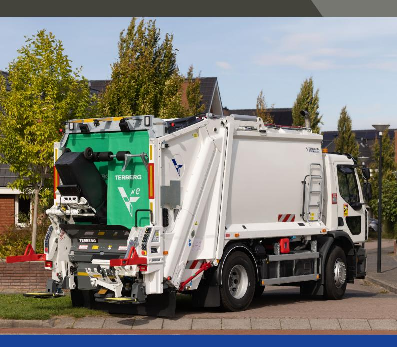
The Terberg OmniMAX\*e has been developed from the ground up to integrate perfectly with our Olympus RCV body. The OmniMAX\*e provides the same superb waste & recycling collection solution as the regular hydraulic version but with the benefits of a low voltage, low noise electric bin lift system. The system has the flexibility to safely handle an impressive range of containers with its robust rear mounted electric lift system. With maximum operational flexibility in mind.
