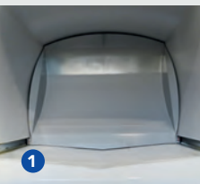
1 Leachate tank at the bottom of the body. Keel shaped floor helps leachate flow to drain sump.
